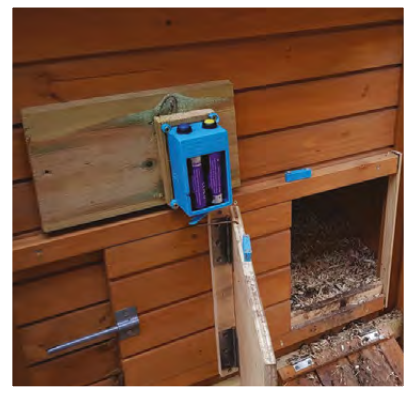
Above ♦ The MK2 chicken door, installed on the coop. The battery cover has been removed to show the 18650 batteries inside. This unit is more compact and much easier to set up
