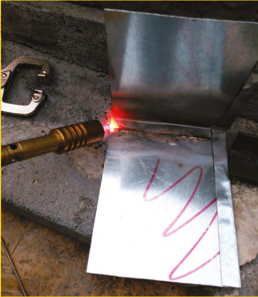
Above ♦ Aim for a dull red or orange colour
