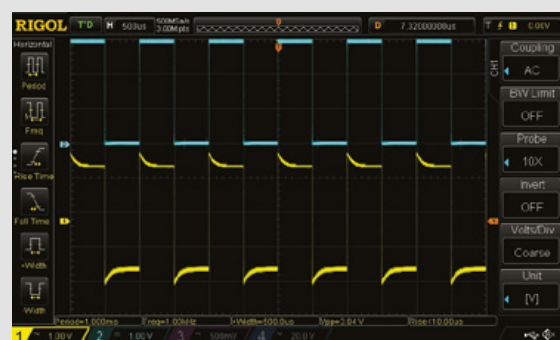
Above ♦ Two identical waveforms; the top one is displayed through a correctly adjusted probe, while the probe carrying the bottom one needs some attention
