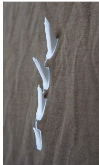
Above ◆ These edgy spikes could easily be used for cosplay. The printer had no trouble printing high 3D shapes directly onto fabric
