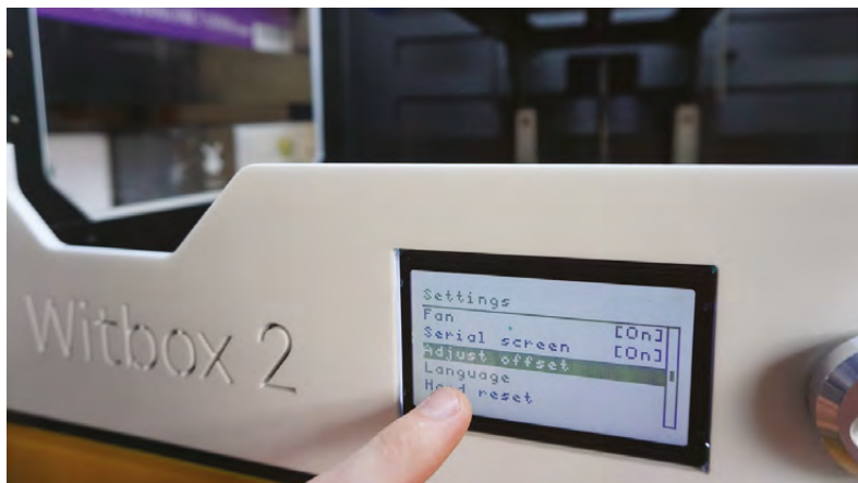
Below ■ You can usually find the 'Adjust offset' feature in your 3D printer's settings
