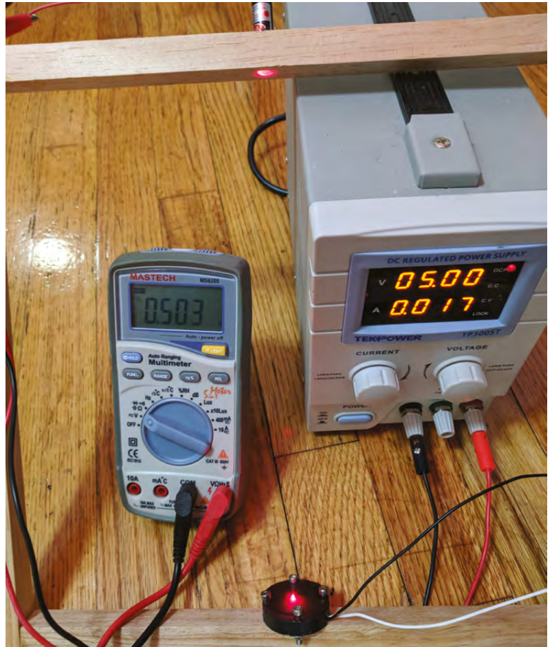
Above ♦ You can test the trip wire by connecting the laser to a 5V power source and reading the voltage off of the solar cell with a multimeter
