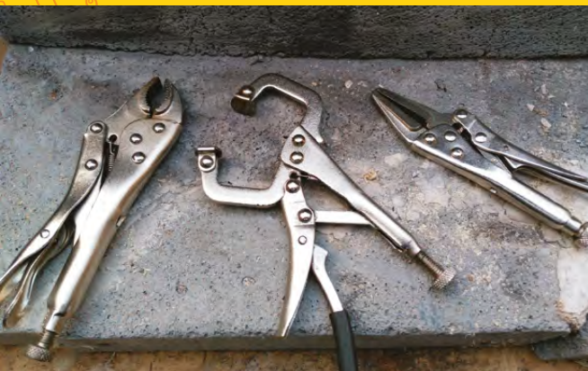
Below ♦ Choose a suitable size and shape of clamp
