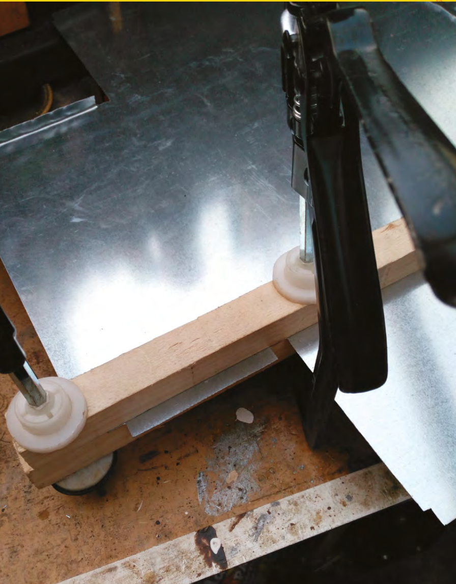
Above Fold against the wooden former
