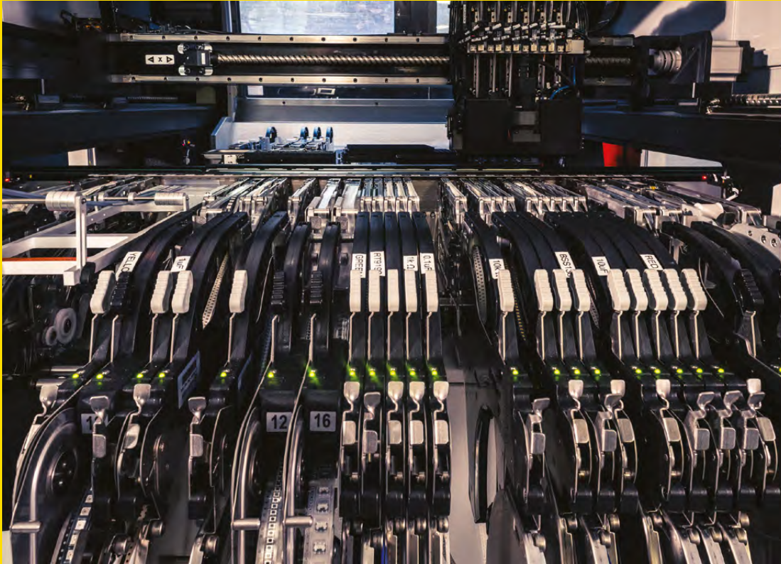
Left ♦ Reels of components waiting to be loaded into the Pick and Place
