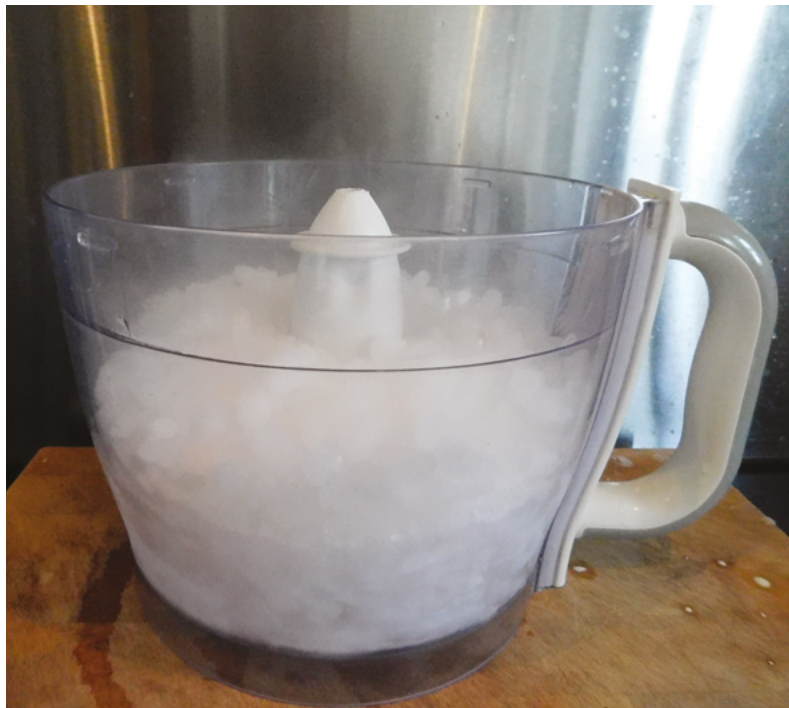
Above ♦ An ordinary food processor will crush dry ice pellets to a fine powder
