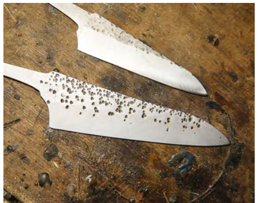
Below ♦ The forge marks on each knife are different every time, and reduce suction when cutting through food
