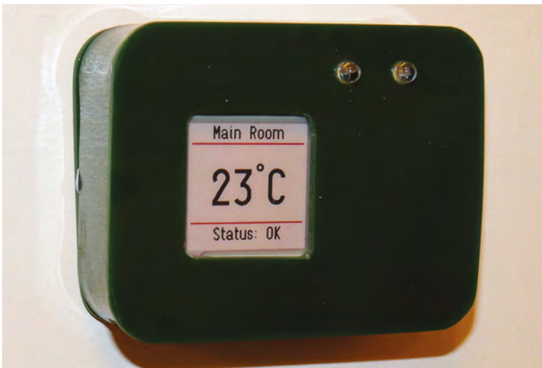
Left The low-powered e-ink display shows temperature data
