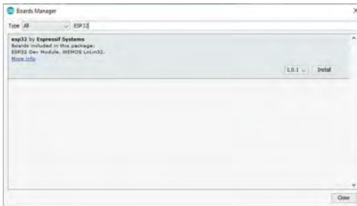
Above ♦ Download the tools and libraries to compile for the ESP32 module
