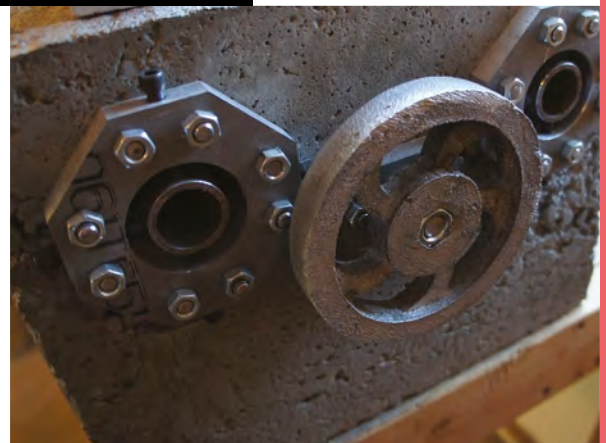
Left ♦ The aluminium plates bolted to the concrete base seen here are used to centre the round pipe for the lathe's DIY linear rail
