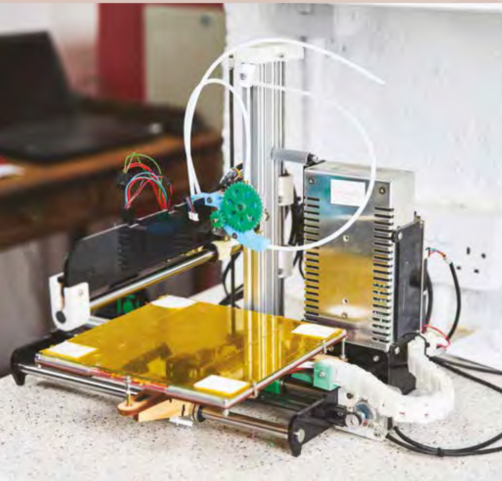
Left This RepRap model, Ormerod 2, is the basic model on which the prototype Arduino-controlled printer is built
