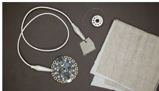
Above ♦ You can test out the fabric with crocodile clips
