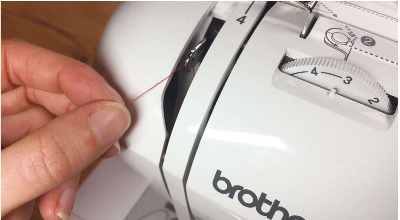
Figure 3 ♦ Make sure the thread take-up lever is at the highest position when threading
