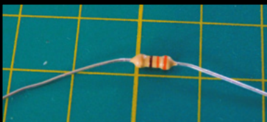
Left The humble resistor allows us to use delicate components without pushing too much current through the circuit
