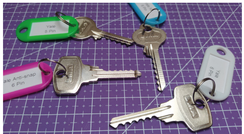
Figure 10 A collection of commercially bought bump keys that fit a range of Yale-style keyways
