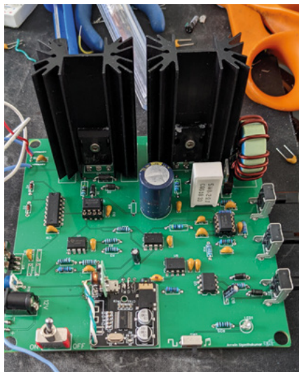
Right ♦ This PCB Tesla coil can create arcs up to three inches long
