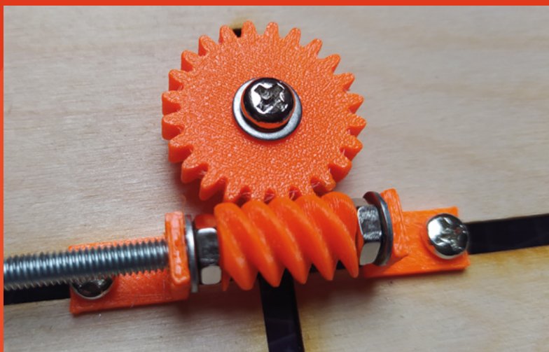
Figure 12 ◆ A 3D-printed worm gear and an involute gear generated in FreeCAD
