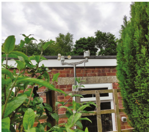
▲ Our weather station's cables go into the garage where a Weather HAT-equipped Raspberry Pi is located – an external weather-proof box would be better, however
