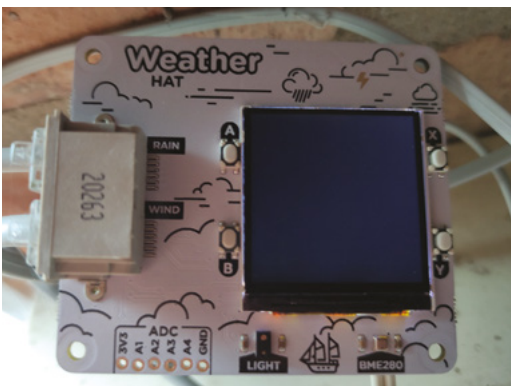
▲ Mounted on a Raspberry Pi Zero (hidden beneath), the Weather HAT has on-board BME280 and light sensors
