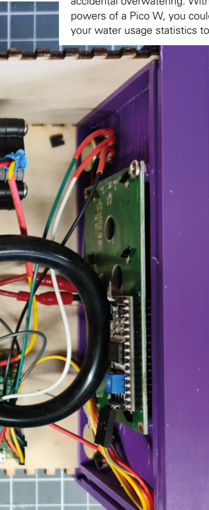
Left □ You can see that the water pump is positioned so that the inlet and outlet connectors are as far away from the panel-mounted quick connectors as possible. This extra distance helps to prevent kinks in the pipe that might restrict the flow
