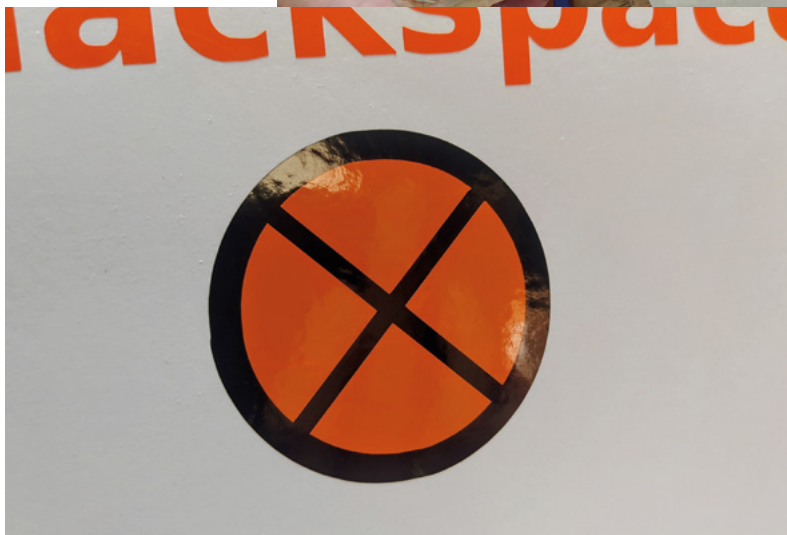
Figure 7 ♦ Using sticky-back vinyl to create a screen print simplifies the screen printing process, and makes the screens last longer and easier to reuse
