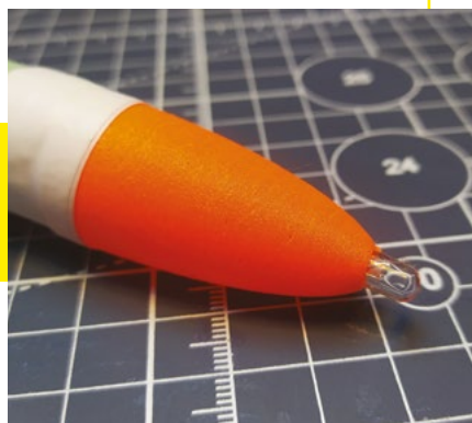
Left A simple nose cone with a fast-blinking LED glued into the tip for night flying
