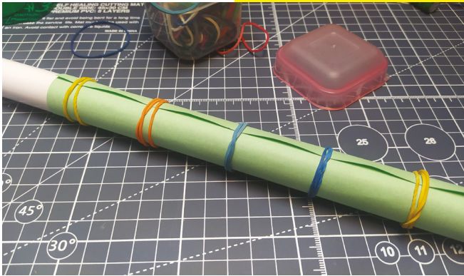
Figure 4 ↑ Using a section of 21.5mm pipe, with a strip of tape added, to create a good-fitting rocket tube
