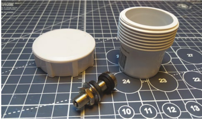
Figure 2 ⬆ A threaded Schrader-style valve with rubber seals
