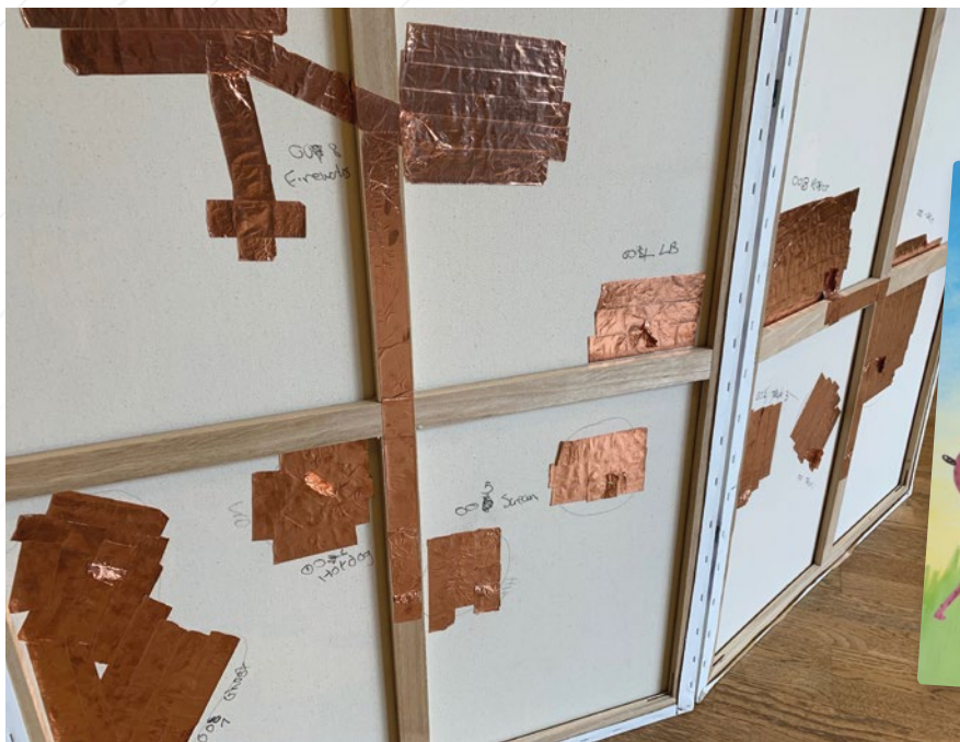
■ The back of the canvas shows the copper tape used to create a conductive surface
