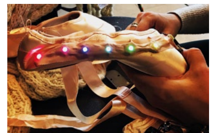
■ Ballet shoes feature Arduino Gemma wearable microcontroller boards and a pressure-sensitive plastic film. Image: ReadySaltedCode CIC
