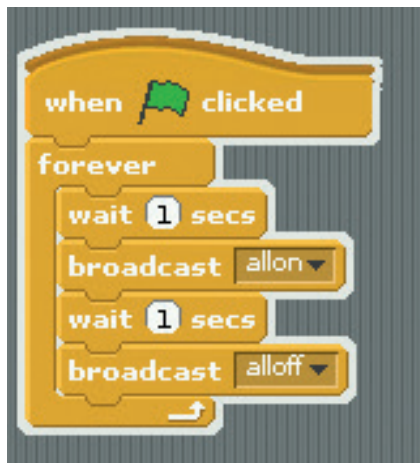
The first circuit simple switches the output on, waits one second, then switches it off, then waits one second and repeats.
