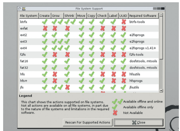
This panel shows the range of filesystems that are supported, and operations available for them.
