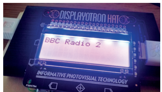
The Displayotron's six touch-sensitive buttons will even work through acrylic, enabling projects to be enclosed.
