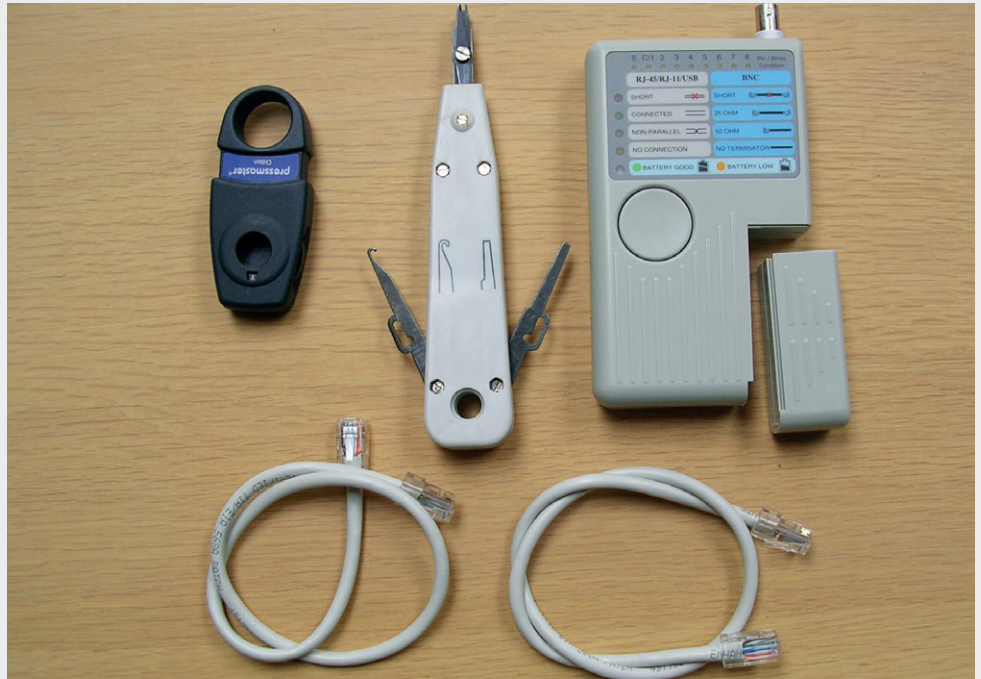
Insulation stripper, punch-down tool, Ethernet tester and a couple of short patch leads. This kit cost less than £20 but is invaluable for installing and testing a wired network.
