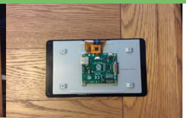
Lie the board on the back of the display and connect the small ribbon to the J4 port.
