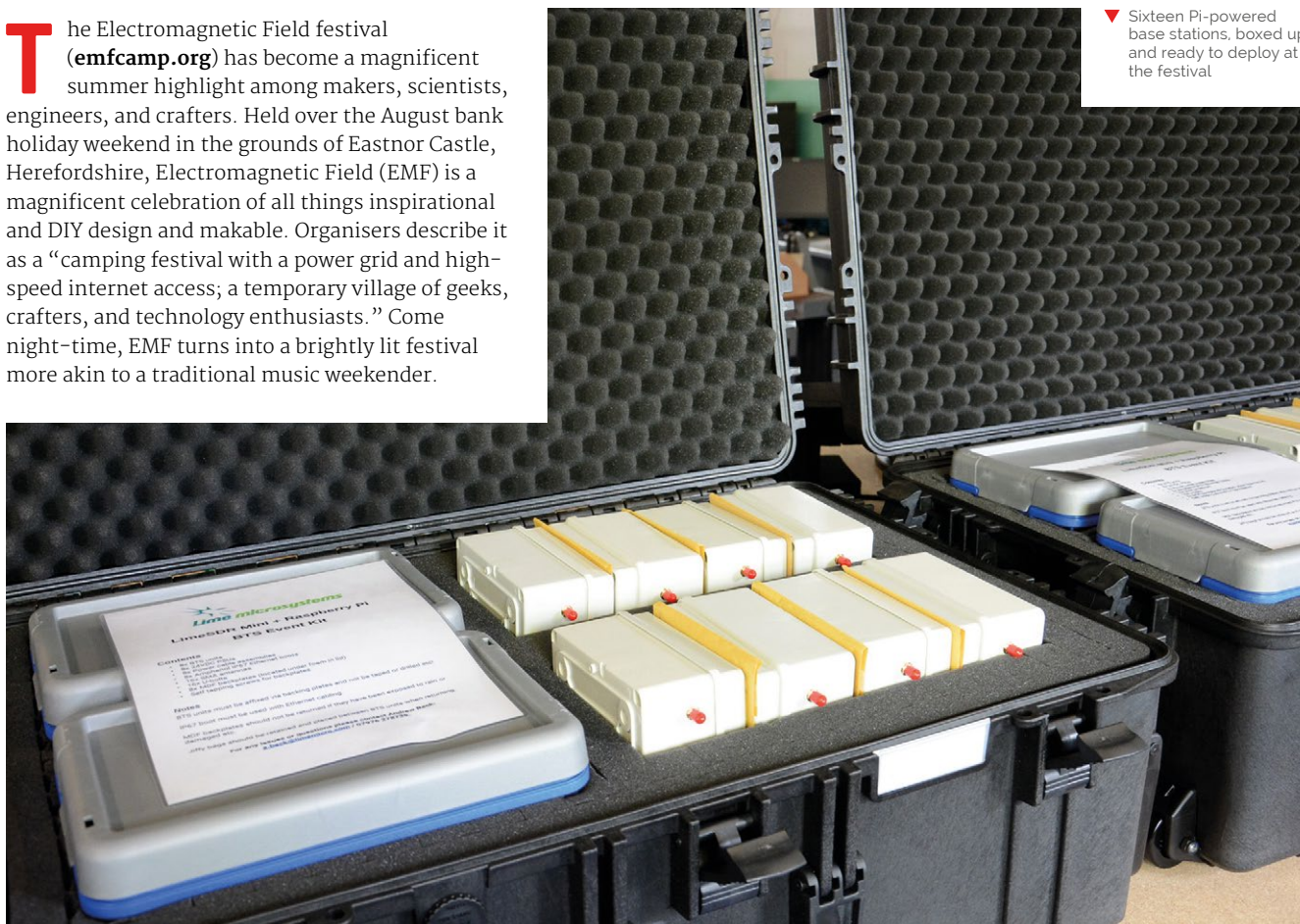
▲ A LimeSDR mounted base station providing GSM for EMF festival-goers
