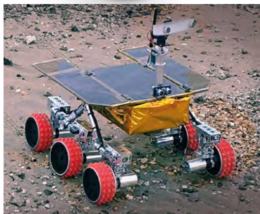
▲ Yuri 3 being tested on a beach to recreate challenging terrain navigation
