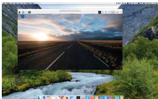
▲ The pre-installed VNC server streams the Pi's desktop user interface to any other computer on the network
