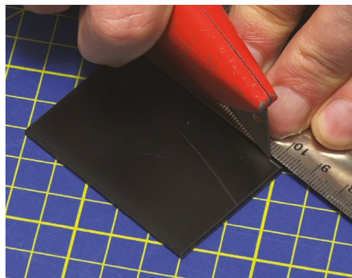
▲ Christopher made his own pods by cutting and pasting together five plasticard pieces for each
