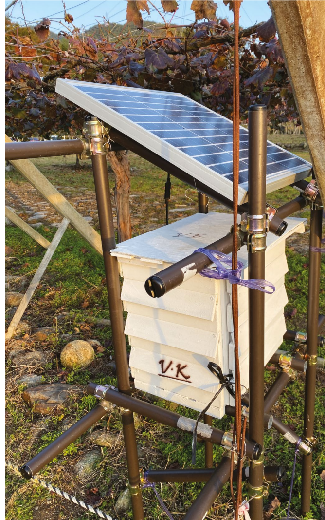
▲ The first prototype system set out in the field. Sensors hang out of the box to obtain an accurate reading
