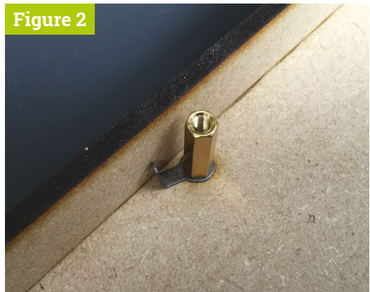
▲ Figure 2 Using a bent solder tag to push out the sides and stop them bending
