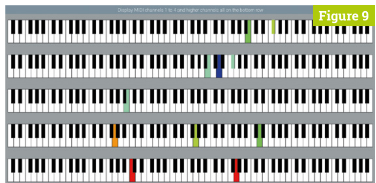
▼ Figure 9 Five keyboards showing MIDI note messages being sent on different channels
