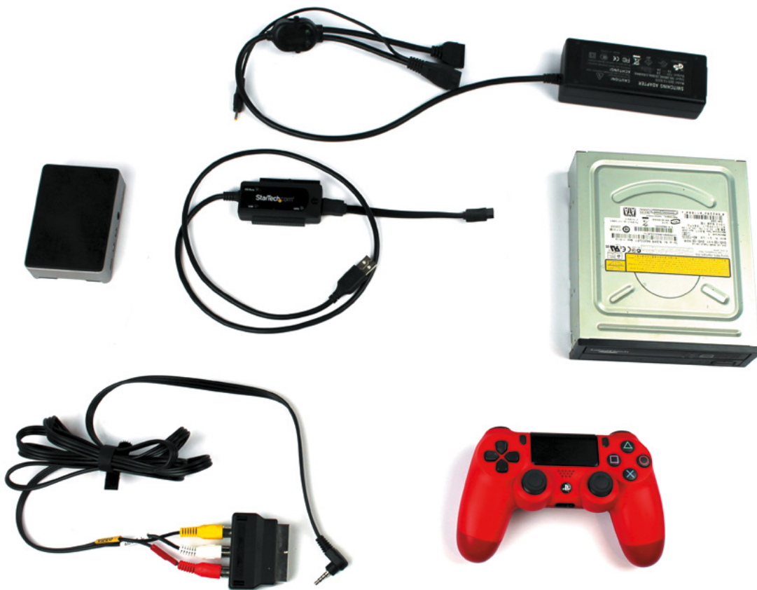
▲ This build included an internal PC DVD-ROM drive, an externally powered SATA-to-USB adapter, a composite video out cable and SCART adapter, a heat-sink case, and controller
