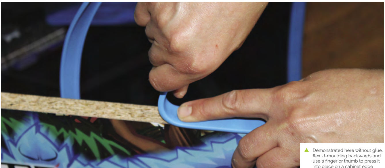
▲ Highly flexible, U- and T-moulding are used to give a clean finish to the cabinet edges
