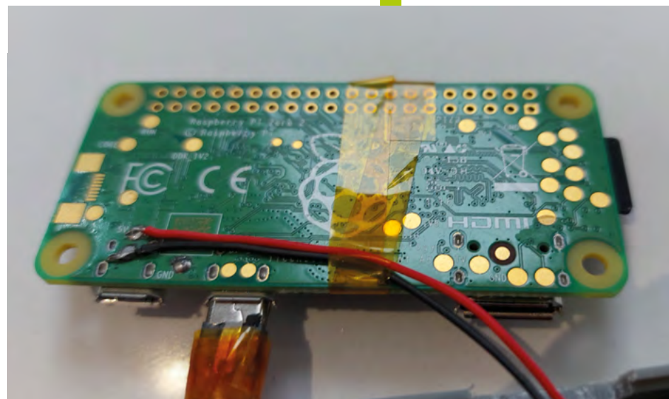
✓ Figure 8: The 5 V and ground wires can now be soldered to the respective pads on the Raspberry Pi Zero 2.
