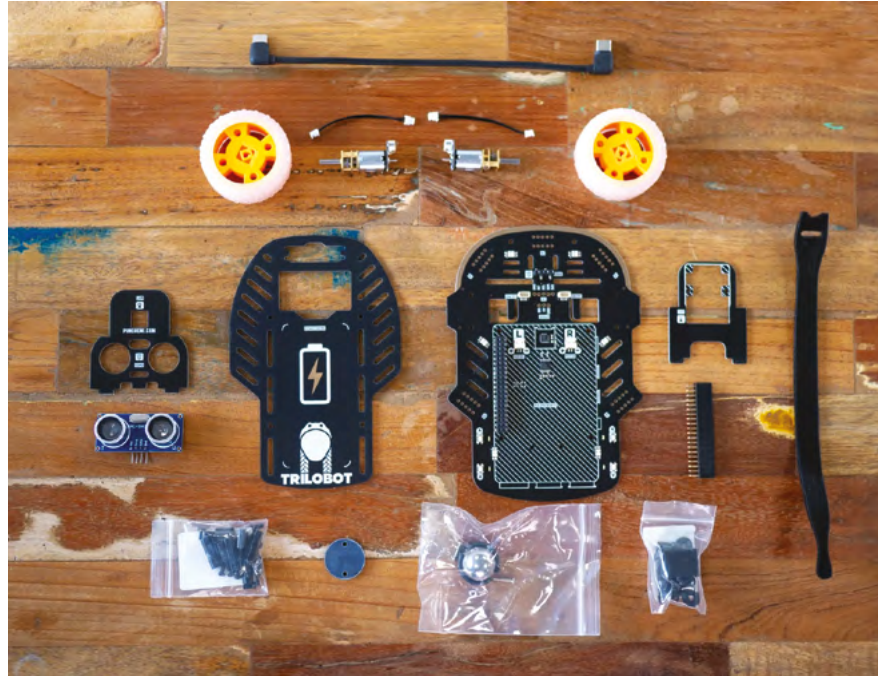
▲ The components supplied in the Trilobot Base Kit. Just add a Raspberry Pi, microSD card, power bank, and Camera Module (optional)
