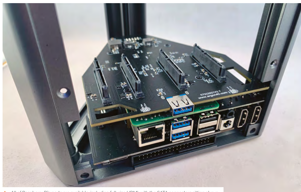
▲ All of Raspberry Pi's ports are available, including full-size HDMI, with the SATA connectors sitting above
