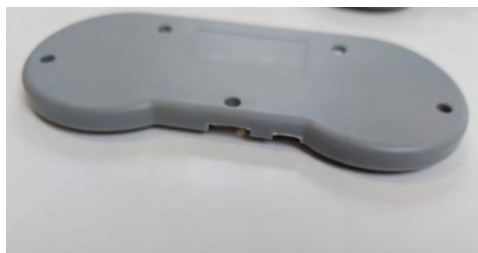
^ Figure 12: Be sure to cut good-sized holes for the on-off switch and the PowerBoost's micro USB port.
