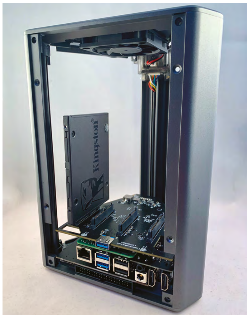
▲ Shown here with a single 2.5" SSD drive. Note the adaptive cooling fan at the top
