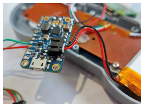
⚠ Figure 9: Ensure the positive (red) and negative (black) wires are the correct way around when you plug your LiPo battery into the PowerBoost.
