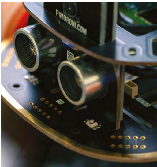
▲ One of the unpopulated Breakout Garden headers is right at the front, although we're not quite sure how practical it is as it's so near to the ultrasonic distance sensor
