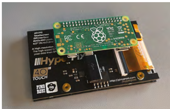
▶ Raspberry Pi Zero will connect directly to the back of the HyperPixel 4.0 four-inch display
