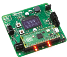
▲ The BME688 sensor is at the top left of the board; its readings can be shown on a small OLED in the middle
