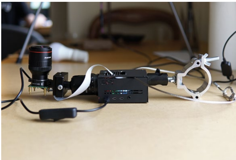
▼ The tracking system uses an HQ Camera and hangs from the ceiling
