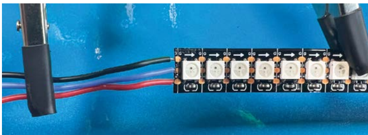
▲ Figure 5 Soldering the wires onto the LED strip
