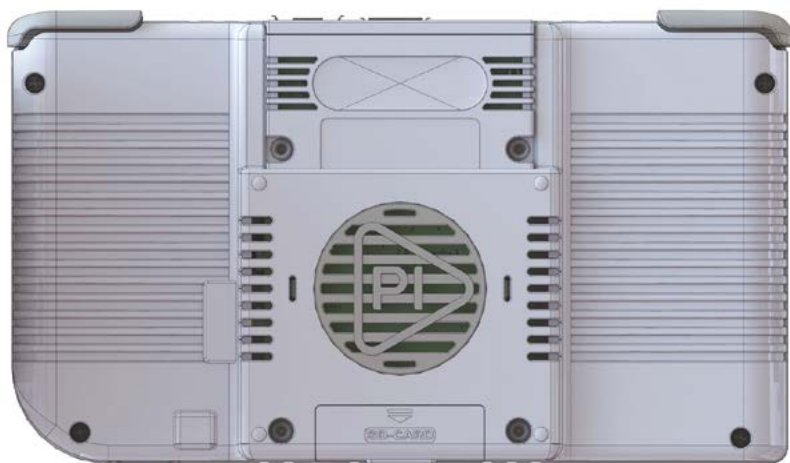
▲ There's easy access to the microSD port, and plenty of ventilation for Raspberry Pi 4 too
