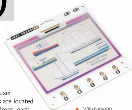
▲ With 640×400 pixels packed into a 4-inch screen, the Inky Frame has excellent definition for displaying images
