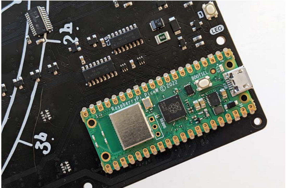
▶ As Raspberry Pi Pico W is on board, there's no need to solder any headers
