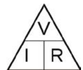
▲ Figure 3 The Ohm's law triangle, makes it easy to find the formula for calculating resistance, voltage, or current
