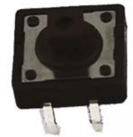
▲ Figure 6 Many switches have four pins. The pins on each side are connected together, with the switch going between them
