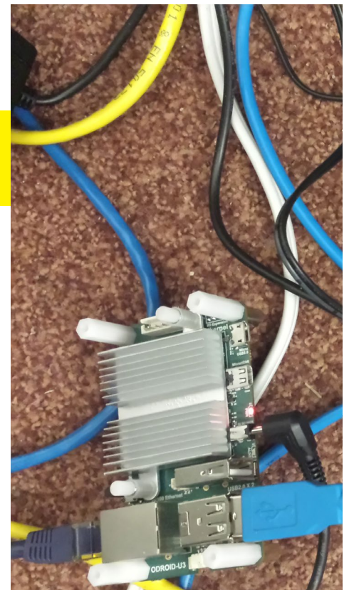
The power use logging setup using an ODROID-U3
