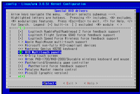
Configuring the touch screen with an embedded driver in the kernel configuration.
