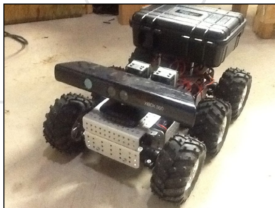
In an earlier development prototype, the UGV used an XBOX 360 Kinect.
