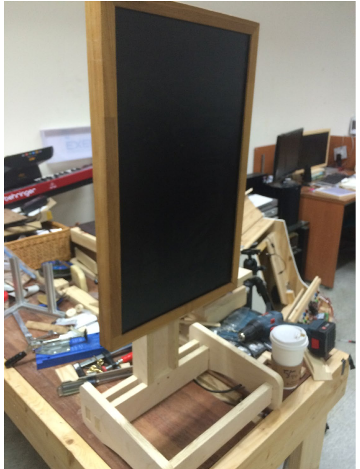
Mount the display unit on the main frame
