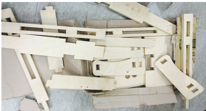
Wood parts by CNC machining
