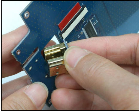
Figure 6 - Plug the HDMI dual gender board to the converter board. It is easier to fit the HDMI dual gender board with this angle
