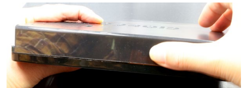
Figure 28 - Press the side of the bottom case together reasonably hard to hook the locking parts
