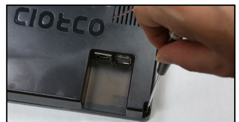
Figure 29 - Insert and tighten the screws on 4 corner side of the screw hole
