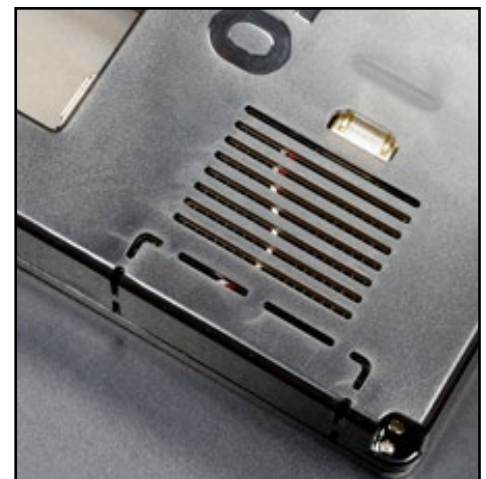
Figure 4 - Vent hole and cutting line for the 40pin GPIO port
