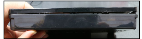
Figure 27 - Close the case. Make sure not to damage the fragile FPCBs and system inside the case
