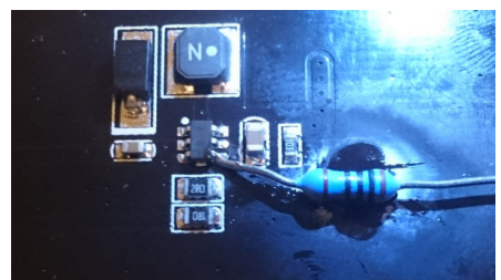
Figure 2 - Closeup of the soldered connection
