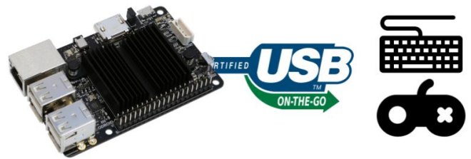
Figure 1 - The ODROID-C2 can act as an HID device using USB OTG device mode
