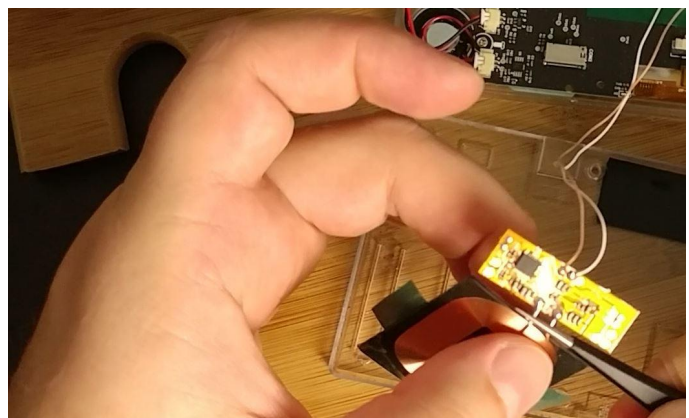
Figure 3 - Bending the Qi coil feed wires
