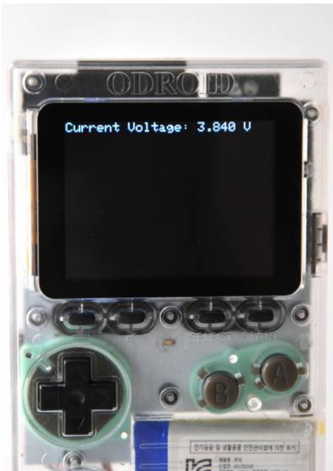
Figure 1 – The ODROID-GO has a ~3.7V battery module
