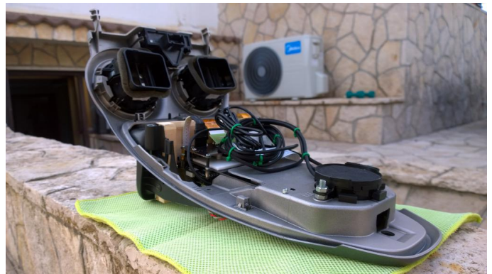
Figure 07 - Underside of Car Dashboard
