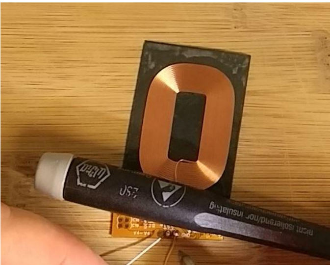
Figure 6 - Adding the wires to the Qi coil
