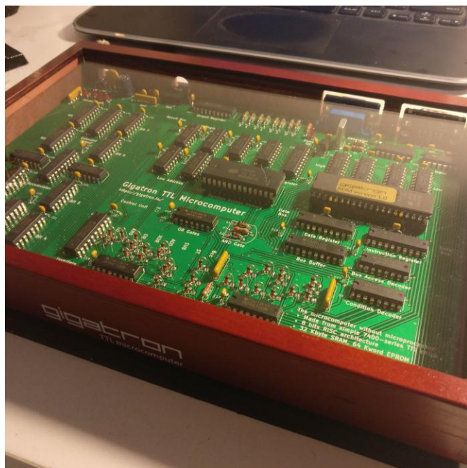
Figure 3 - A finished build of the Gigatron TTL microcomputer
