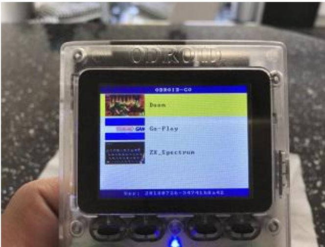
Figure 1 – Place .fw files in ODROID/firmware, then turn off, hold B, turn on and wait holding B until menu appears
