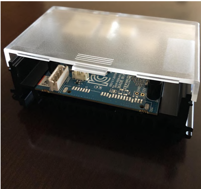
Figure 4 - Just leave the back door open on your build farm for keeping the ODROID-MC1 Solo cool while handling all of its chores.
