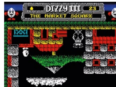
▲ Figure 5: Fantasy World Dizzy's market square, which flipped the sprites by adjusting the values in lookup tables.
