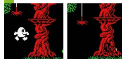
▲ Figure 6: Fast, easy, XOR sprite printing as used in the original Dizzy game.
