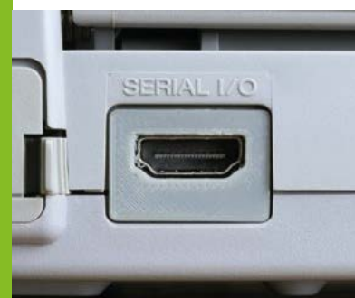
✓ The community pushes for 'no-cut mods' wherever possible. PS1Digital occupies the Serial I/O port.
