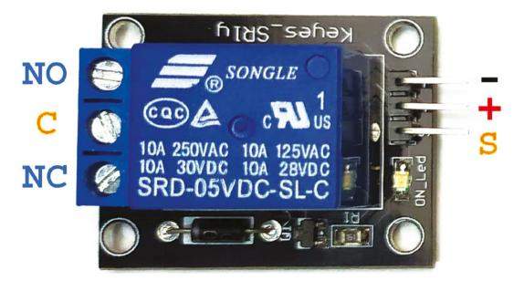
Right ♦ This is the pinout of our relay module, but check yours before wiring it up. You may need to adjust our wiring to match your module. the circuit and return to the original state, it needs an impulse low
