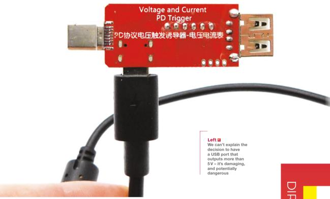
The first thing to say about this board is that the output is via a regular USB port, but it outputs the full voltage from USB-C PD (up to 20 V). In other words, DO NOT PLUG ANYTHING INTO THIS **USB PORT THAT IS EXPECTING A STANDARD** USB VOLTAGE. You will damage it, and you might set it on fire. Why the designers chose this as an output connector, rather than having a barrel jack, is
