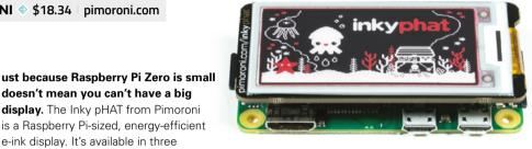
battery will last a long time compared to a traditional LCD or TFT display. Just keep in mind the refresh of the screen can take up to 15 seconds, so don't expect to run any animations or videos!
