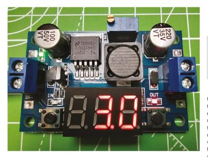
Figure 3 Another variant of the LM2596 board with a switchable LED voltmeter that can show the input voltage and also the variable output voltage
