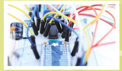
So far, Tim has controlled over 900 WS2812 LEDs using a Raspberry Pi Zero, leaving it on for hours without the board getting warm.
