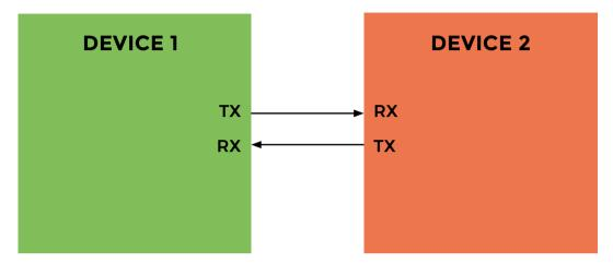
Left Example serial port connection, TX is connected to RX
