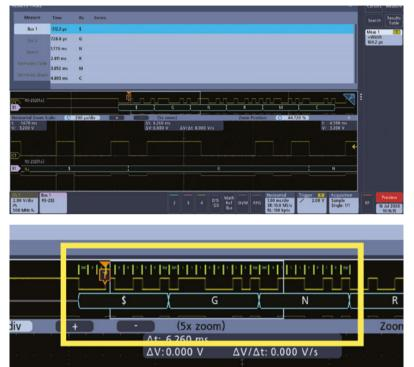
Above Decoding characters from a serial port this can be connected to multiple RX. Being asynchronous, there is no separate clock and the sender and receiver synchronise from the transitions on the data line. Typically, the sender keeps the line high when it is idle.
