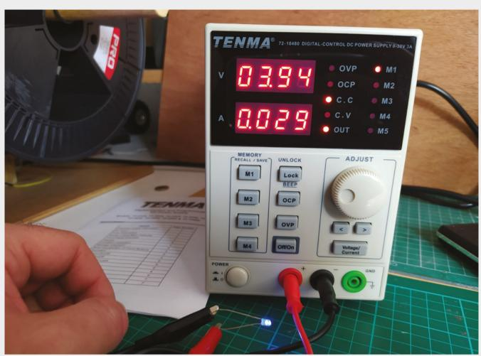
the dial to switch to M5. When any change is made in any memory slot, it's automatically saved. Switching between any memory slot automatically turns off the output, so you can't accidentally fry something by switching to a different supply.
