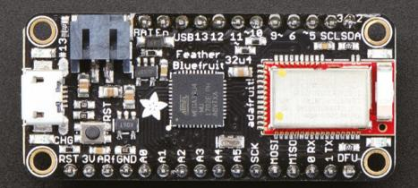
Adafruit's Feather 32u4 Bluefruit was the very first Feather created. The board is wide enough to accommodate a Bluetooth module, yet still narrow enough to fit comfortably on a breadboard. It has space for plenty of IO and a LiPo charger. This format proved so useful that many more followed, both from Adafruit and others, and it's now one of the dominant ecosystems for makers. This month we're celebrating Feather in all their forms.
