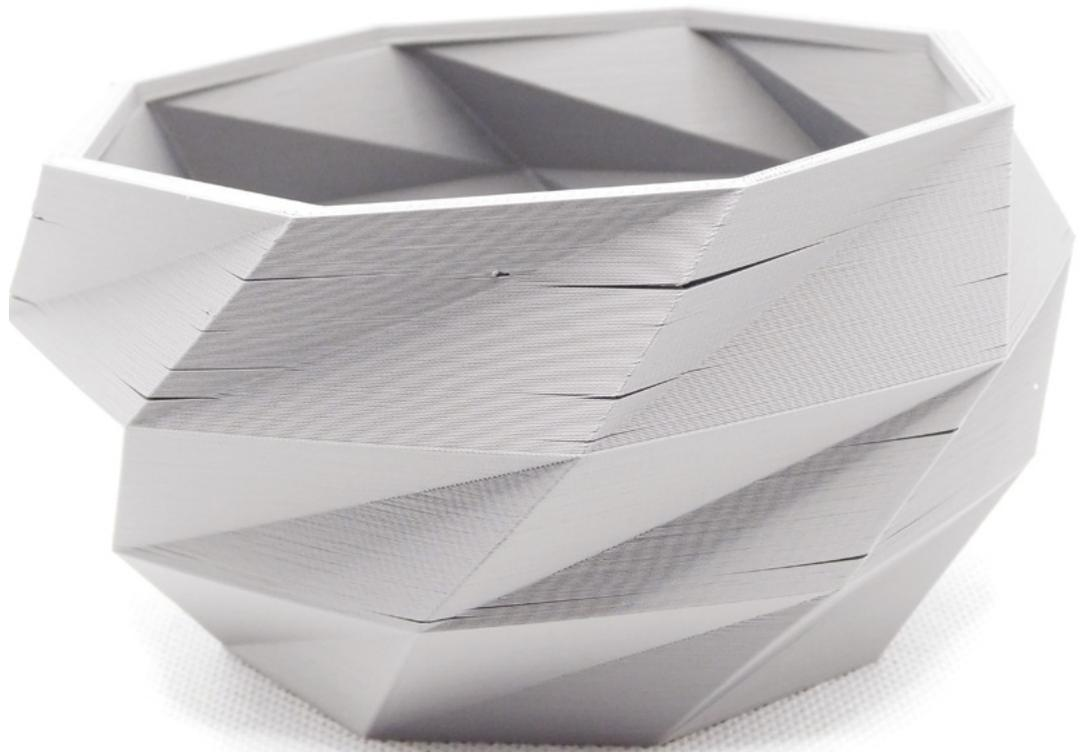
**T**he big selling point of ASA is its weather-resistance. You can print bits with this plastic, leave them outside, and expect them to last. Other 3D-printable materials are prone to breaking down with UV exposure. It's also more temperature-resistant than most common 3D-printable filaments, which is an extra bonus for anything that might be exposed to both UV and heat like something on a car dashboard.
