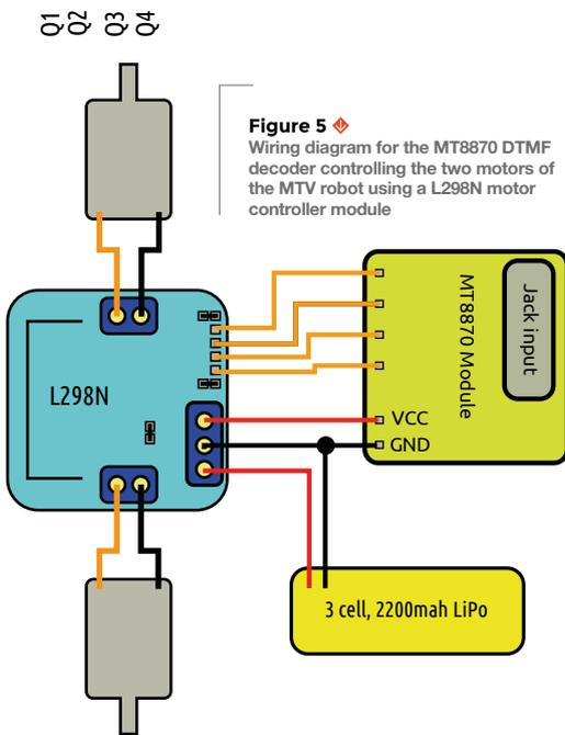
**Figure 5** ♦ Wiring diagram for the MT8870 DTMF decoder controlling the two motors of the MTV robot using a L298N motor controller module
