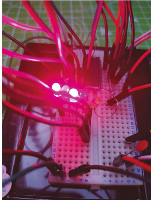
**(Figure 4).** We made an input for this circuit by connecting a 3.5mm stereo jack socket with the right channel connected as input – we then used an audio cable to attach the breadboarded circuit to our mobile phone headphone socket. We turned everything on and then tapped some keys on the keypad of our mobile phone to generate some DTMF.
