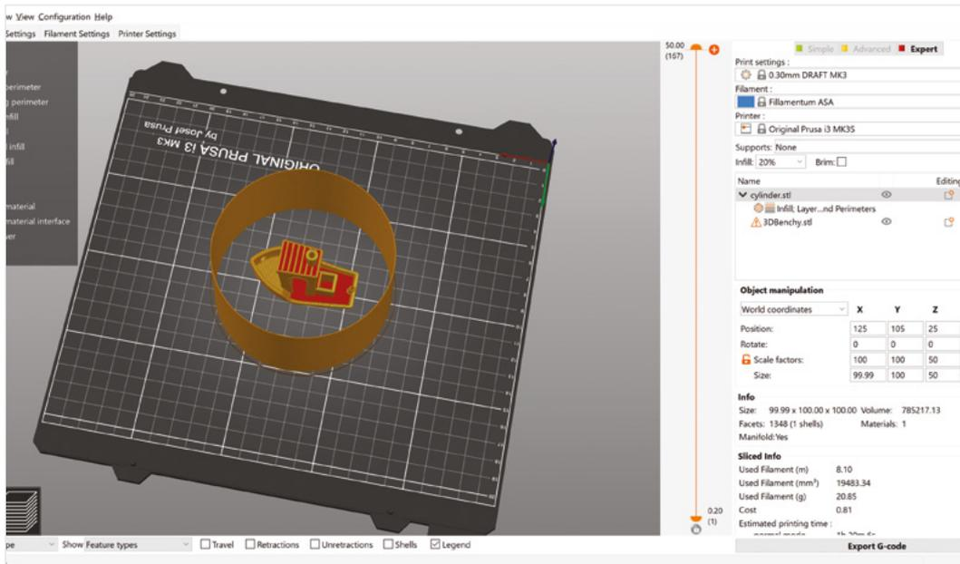
**Left** ♦ When printing without an enclosure, you might have better results if you put a cylinder around your object to stop it cooling too quickly
