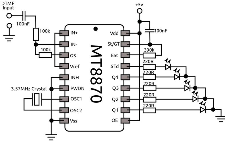
The 4-bit outputs from a receiving end of a hardware DTMF system are at logic level, so it means that we can use these 4-bit words to interact with other hardware.
