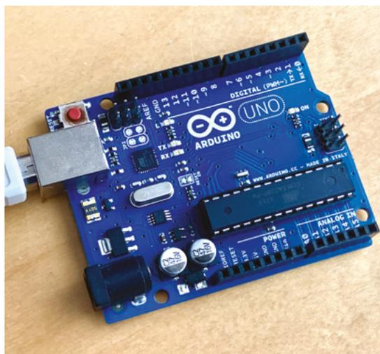
**Left** ♦ A straightforward USB cable is by far the easiest way to connect an Arduino to Raspberry Pi
