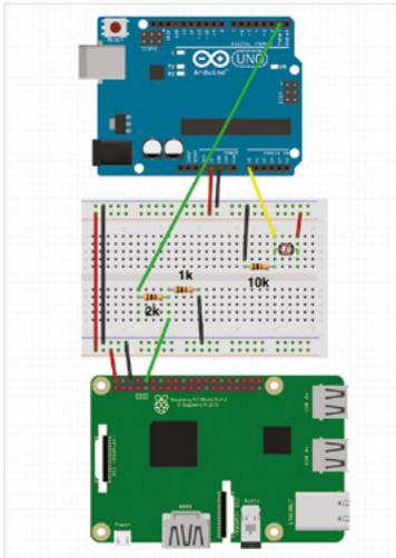
**Figure 2** ♦ A voltage divider lets us connect serial ports
