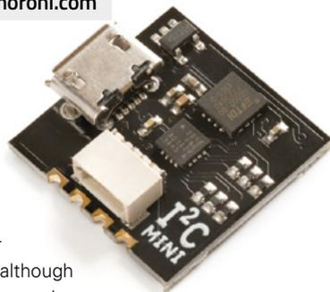
**S**o, what can this little board do? A lot! The I<sup>2</sup>CMini is a USB to I<sup>2</sup>C bridge which allows you to monitor and control I<sup>2</sup>C traffic from your computer or another device. The board, although incredibly small, features a USB connector and a Qwiic connector, along with pins for a breadboard – or simply add some header pins.
