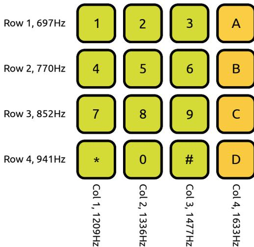
**Figure 1** ♦ The DTMF keyboard layout and the corresponding tones for each row and column
