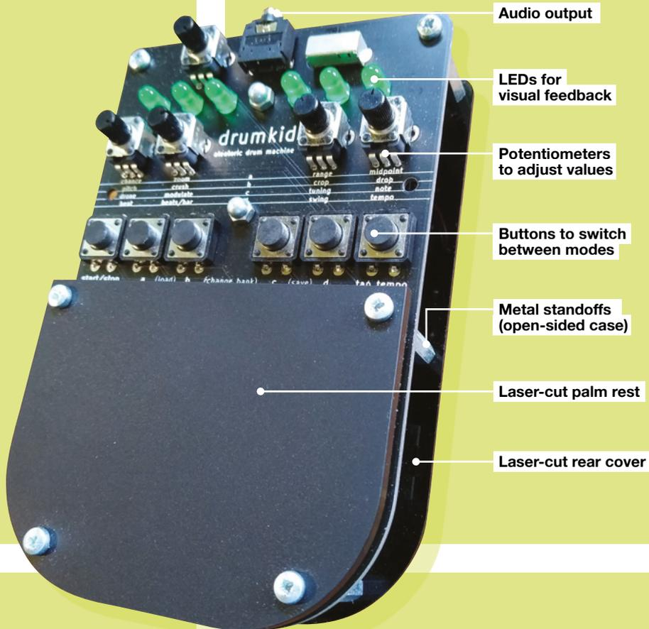
I realised quite early on that 3D-printing would be impractical for the final design, but I decided to print a case anyway, just so that I had a starting point. The aim was to evoke a Game Boy, with LEDs in place of the display and a set of controls for each thumb. The 3D-printed prototype felt comfortable to hold, but was awkward to play because I had decided to only include one potentiometer, so you had to press a lot of buttons before you could adjust the desired parameter.
