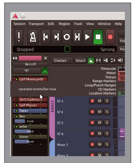
Figure 9: When holding down the Ctrl key, clicking any controller in the mixer with the middle mouse button connects the next incoming controller signal to the current controller. Individual controllers from plugins such as Calf Monosynth can be placed directly in the channel.
