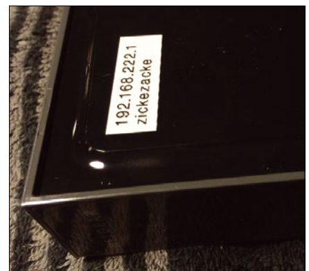
Figure 1: Fast diagnostics thanks to systematic organization: the configured IP address and WiFi SSID on the router.
