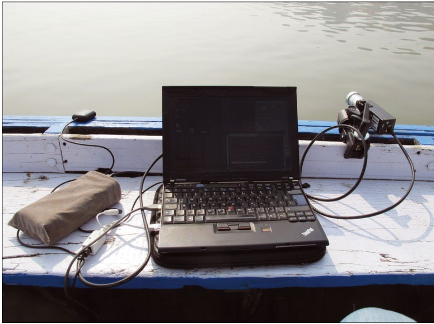
Figure 3: The hardware (from left to right): GPS receiver, bag with batteries, laptop, and camera.
