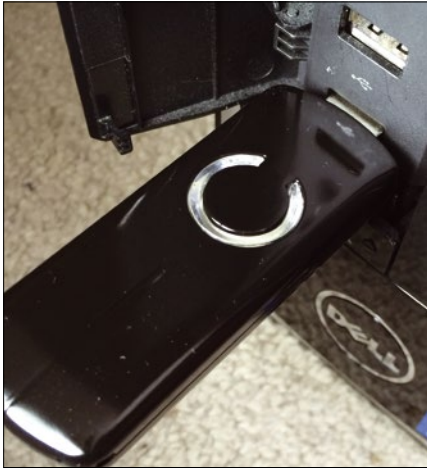
Figure 1: The Z-Stick controller by Aeon Labs for plugging into a PC USB port.
