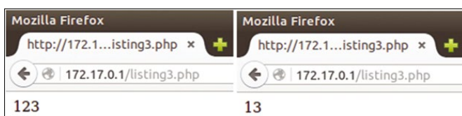
Figure 3: Left: PHP 7 default behavior; iterating over a copy of the $arr field. Right: backward compatibility with PHP 5; iterating over the actual $arr field by using the & character.
