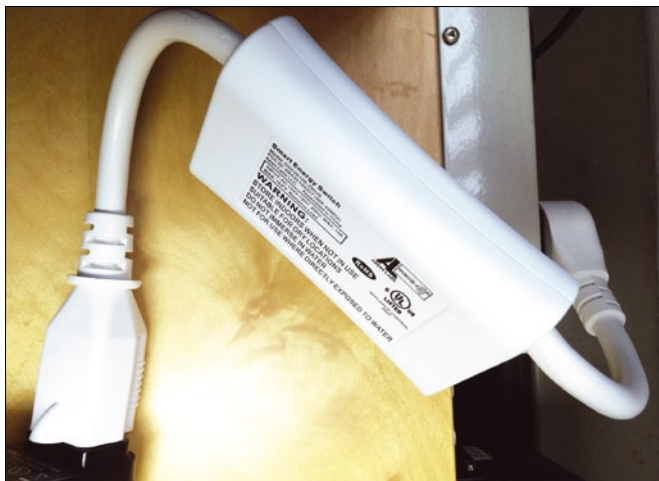
Figure 2: The Z-Wave Smart Energy Switch receives wireless signals and switches electrical consumers on and off.
