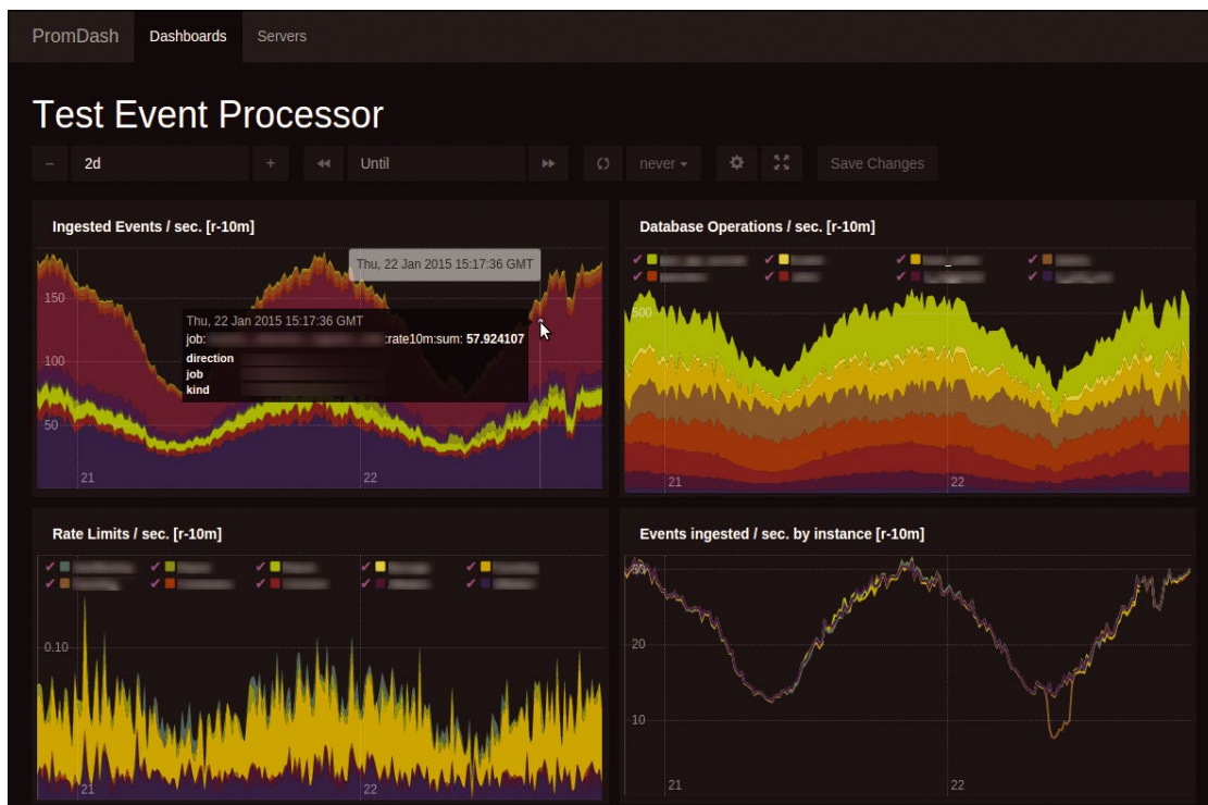
Figure 5: Prom Dash is a helper that lets administrators create graphs based on Prometheus data.
