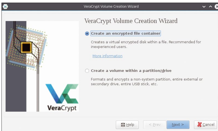
Figure 2: The intuitively designed VeraCrypt dialog lets you create encrypted containers, even without prior knowledge or studying the manual.
