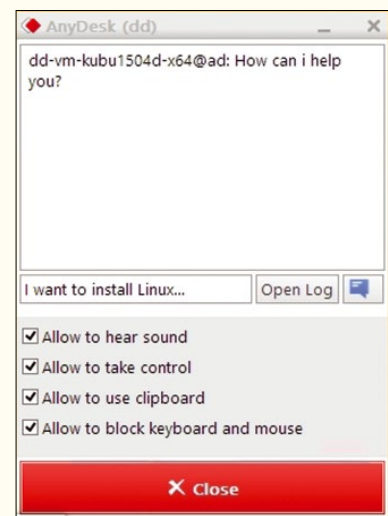
Figure 3: AnyDesk requires explicit approval of the connection setup on the remote computer. This is where the permissions granted are specified.
