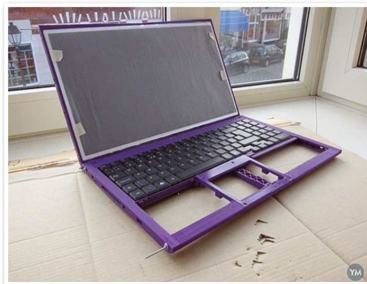
Figure 1: An early version of the laptop showing 3D-printed parts.
