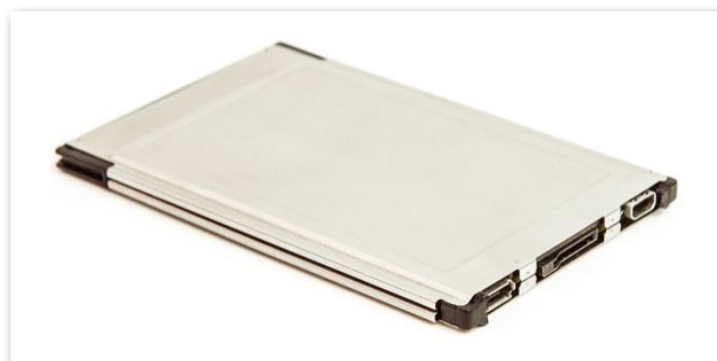
Figure 3: Computer cards slide into the rest of the laptop, allowing quick changes of operating systems. They are housed in recycled PCMCIA cards.
