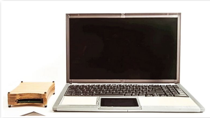
Figure 2: The EOMA68 laptop. Notice the bamboo frame around the screen and the home-made housing for the computer card.
