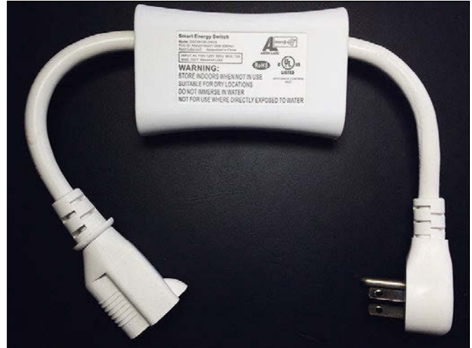
Figure 2: The Z-Wave slave, in the form of the Aeon Labs DSC06106 network switch, receives commands for switching the consumer on and off wirelessly.
