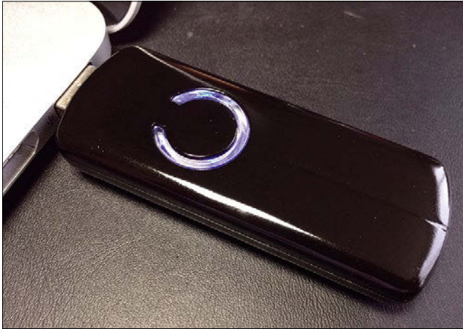
Figure 1: The Z-Wave DSA02203 USB stick controller by Aeon Labs lets a Linux system send wireless commands to Z-Wave slaves.
