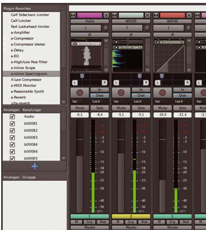
Figure 7: Scope, Spectrogram, and Compressor from the Ardour plugin collection show their output directly in the Mixer tracks.
