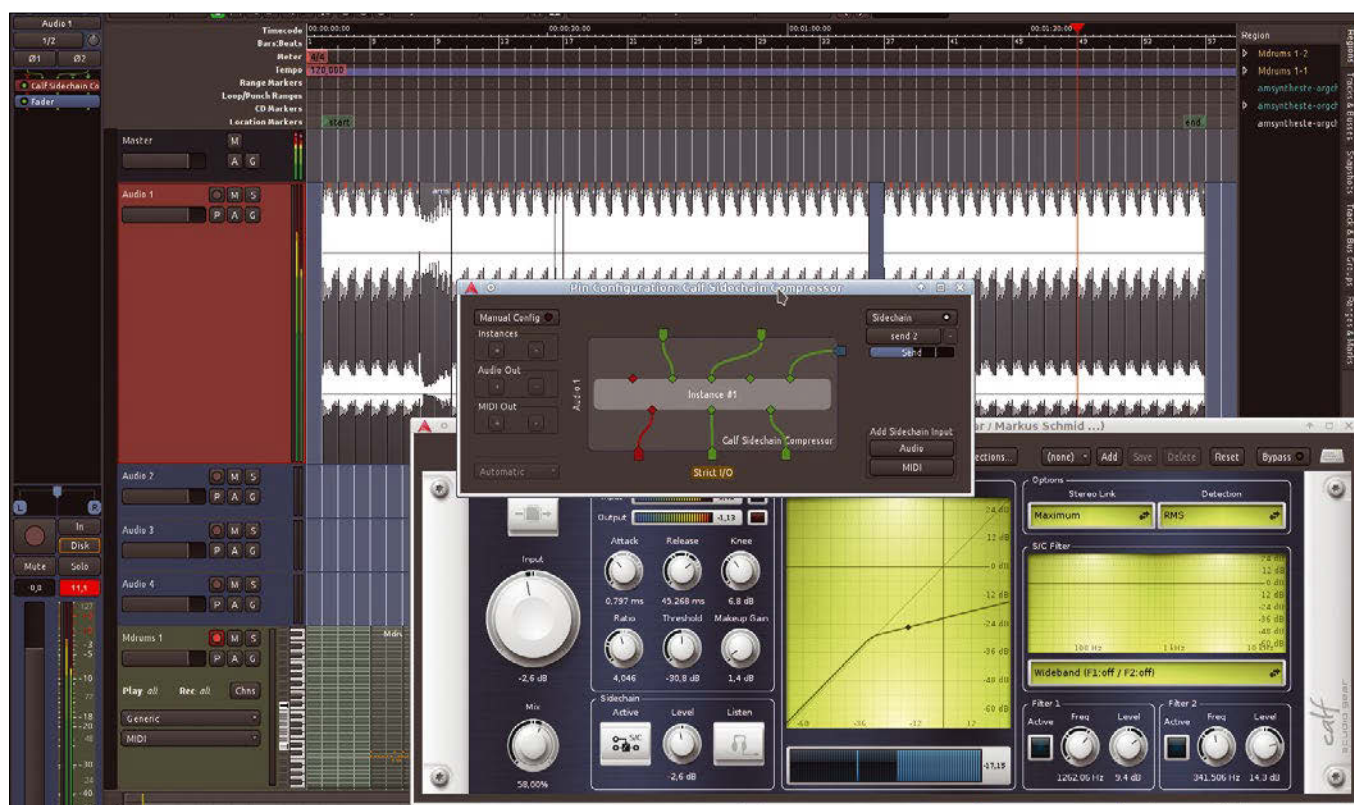
Figure 9: The Calf Sidechain Compressor is ideally suited for creating popular pump effects where the beat of a bass drum rhythmically down-controls a synthesizer section.
