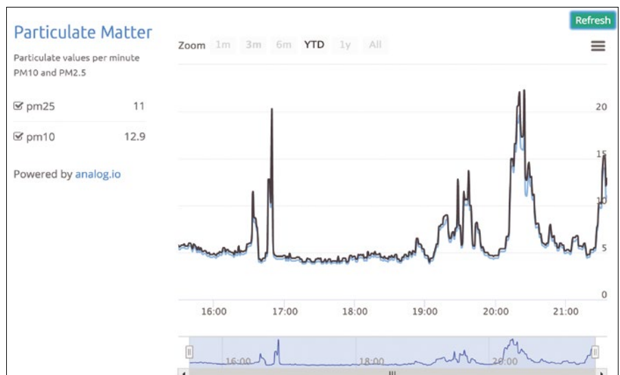
Figure 2: The free SparkFun web service visualizes the readings passed to it.
