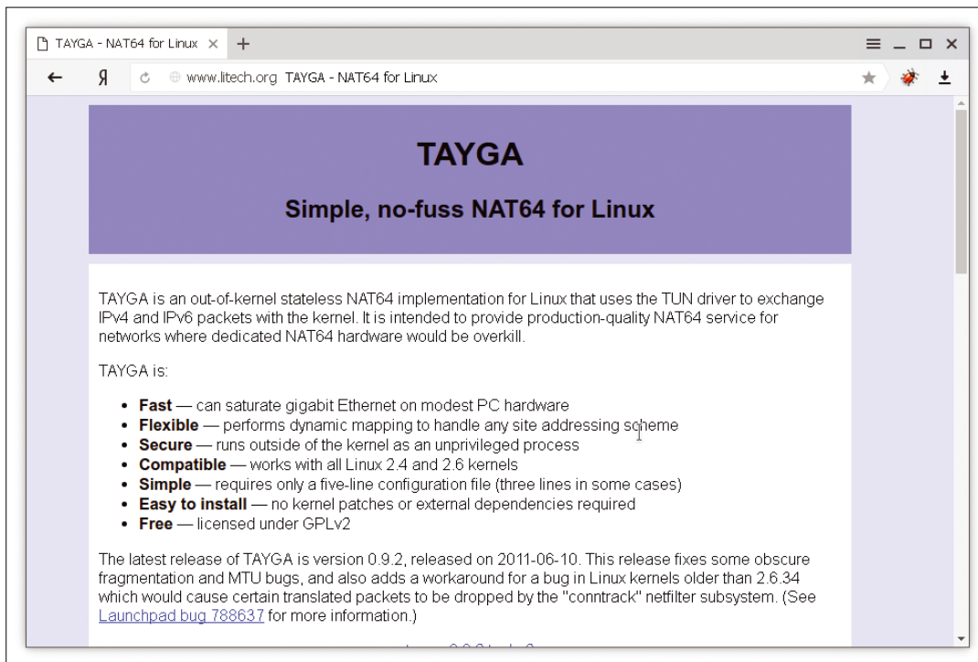
Figure 4: Tayga is a quite popular NAT64 implementation for Linux. Like Miredo, it uses TUN devices and runs in userspace.
