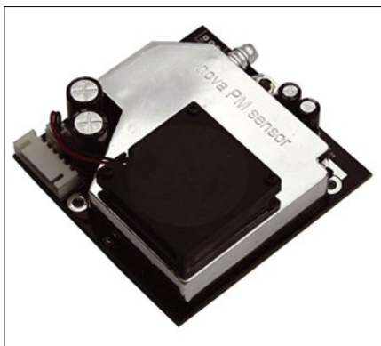
Figure 1: The particulate matter sensor from the Far East that Charly connected to his Raspberry Pi.
