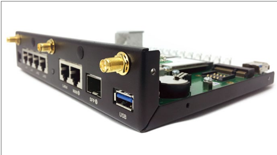
Figure 2: Exotic specimen on the router market: The Turriss Omnia offers five Ethernet interfaces, as well as one Gigabit Ethernet interface, WiFi, and an SFP port. (Source: CZ.NIC)
