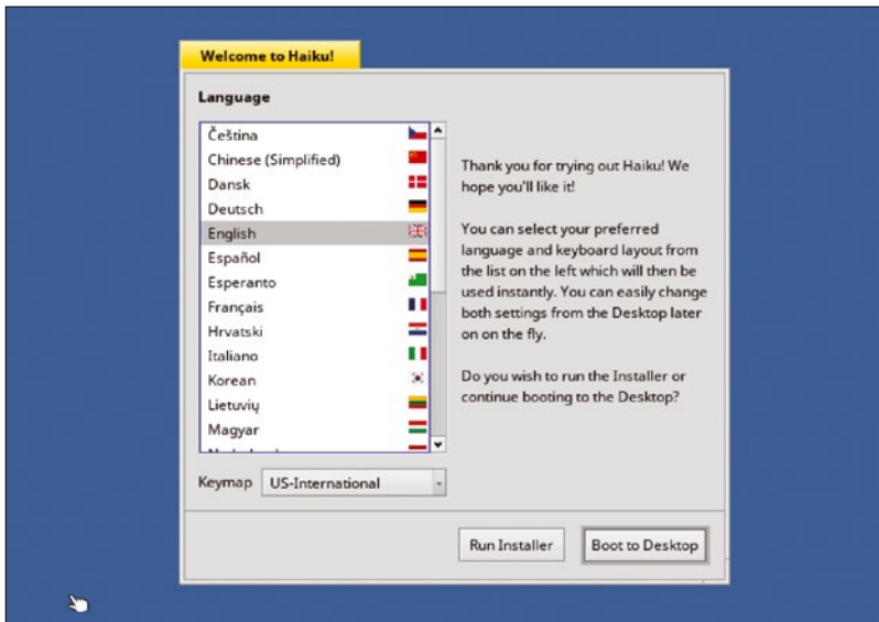
Figure 3: Haiku can be run in live mode from a CD or be installed directly to your hard drive.
