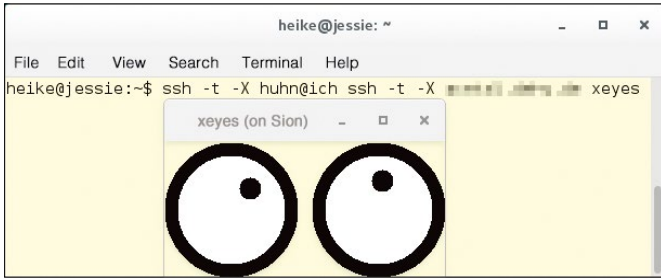
Figure 2: The xeyes program runs on the third host named Sion; however, the display appears in the graphical interface of the first computer (jessie).
