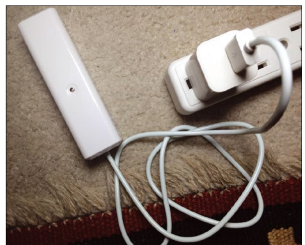
Figure 10: The battery-powered power outage sensor by sevenexpress shows the user whether or not power is available as a door sensor.
