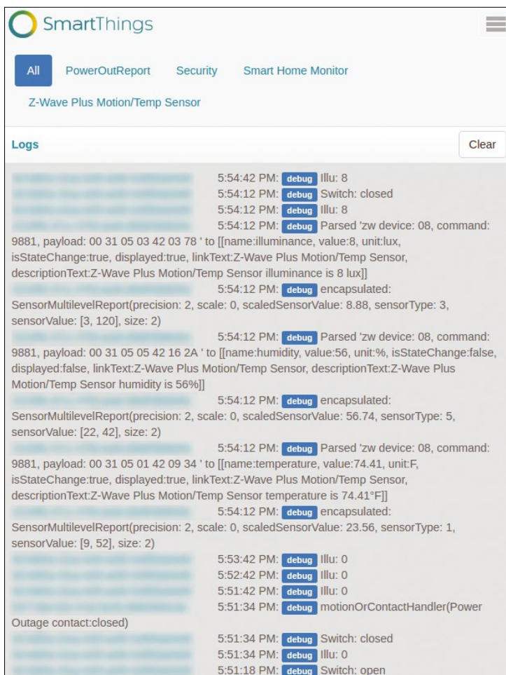
Figure 9: The hub queries the light sensor every four minutes, whereas events on the contact sensor appear immediately.
