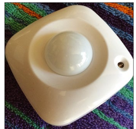
Figure 5: The battery-powered light-motion-temperature sensor by Zooz speaks Z-Wave with the controller.
