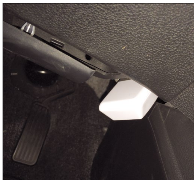
Figure 3: The OBD-II port for plugging in the adapter is usually below the dashboard.
