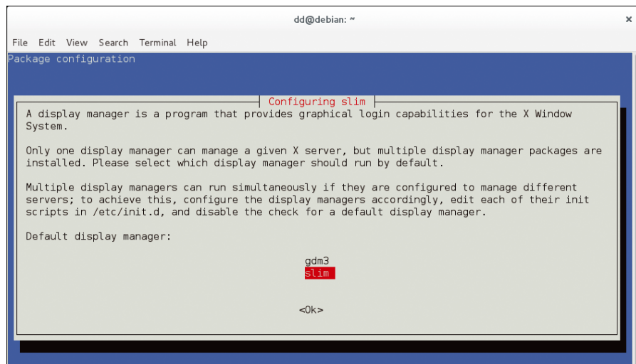
Figure 3: Opt for SLiM, the lean login manager, rather than GDM or KDM.
