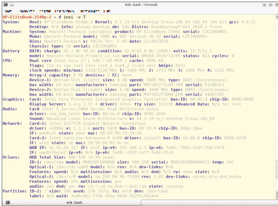
Figure 1: Inxi is visually very plain but technically provides very detailed information about installed hardware.
